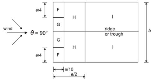
Figure C.8: Wind pressure zones for roof, wind perpendicular to gable [34].
