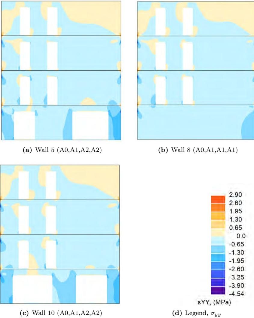
**Figure 4.28:** Walls with opening C and D. Vertical stresses  $\sigma_{yy}$  [MPa].
