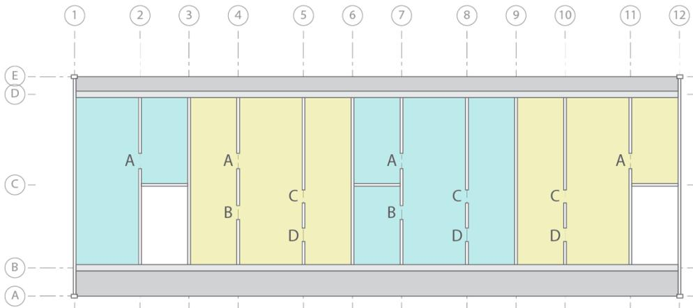
**Figure 4.15:** Existing openings in bearing walls.
