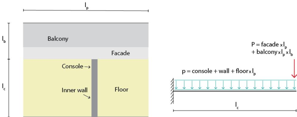
**Figure 4.25:** Illustration of loads for design proposal 3, plan view and cantilevered beam.
