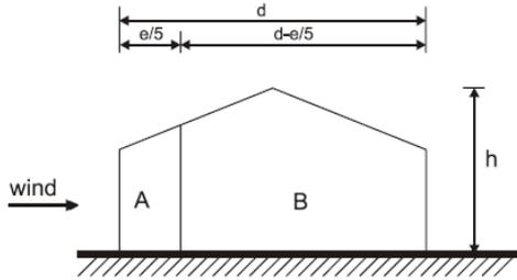
**Figure C.5:** Wind pressure zones for vertical walls,  $e \geq d$  [34], wind perpendicular to facade.
