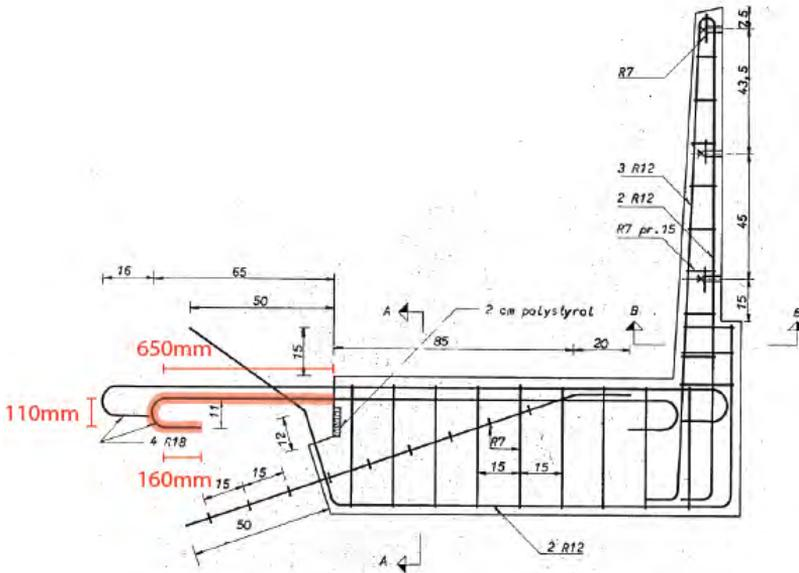
Figure 4.14: Illustration of minimum anchoring length.
