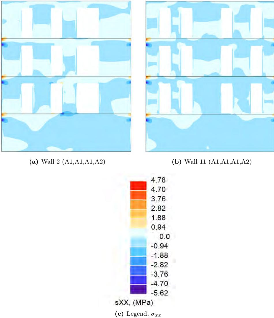
**Figure D.22:** Walls with original opening A, new openings. Horizontal stresses  $\sigma_{xx}$  [MPa].
