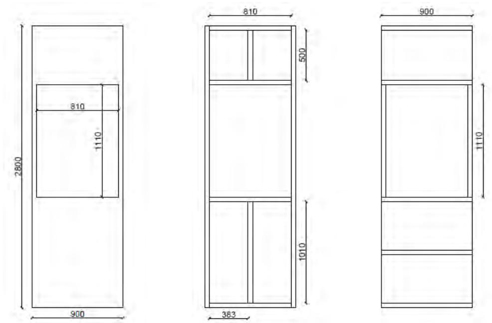
**Figure C.2:** Facade dimensions [mm] for 0.9m element. Wall area, placement of 45x45 timber laths and placement of 200x45mm timber laths.
