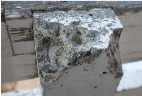
**Figure 3.32:** Aggregates in concrete, block 7.
