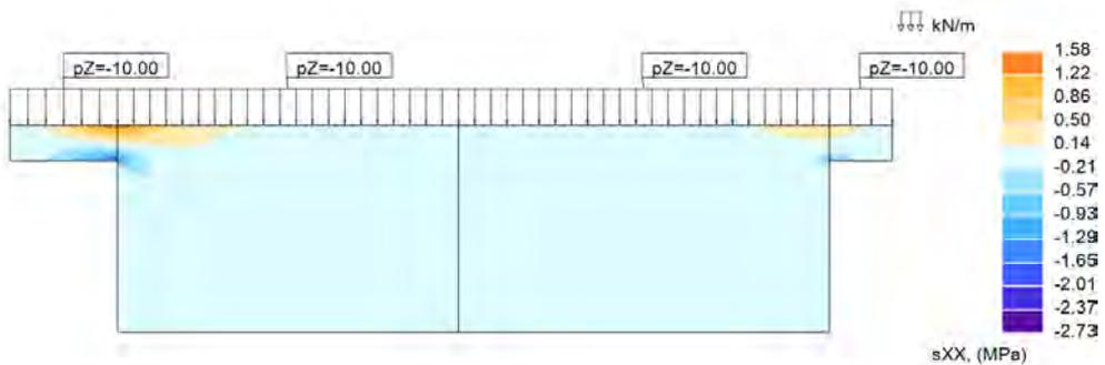
**Figure 4.18:** Illustration of horizontal stresses  $\sigma_{xx}$ . Negative blue numbers = compression. Positive orange numbers = tension.
