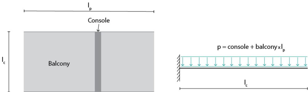
**Figure 4.20:** Illustration of loads for design proposal 1, plan view and cantilevered beam.
