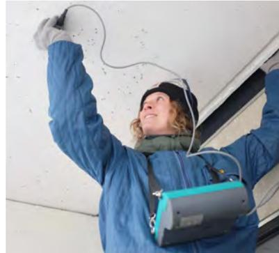
**Figure 3.6:** Measurement of cover layer.
