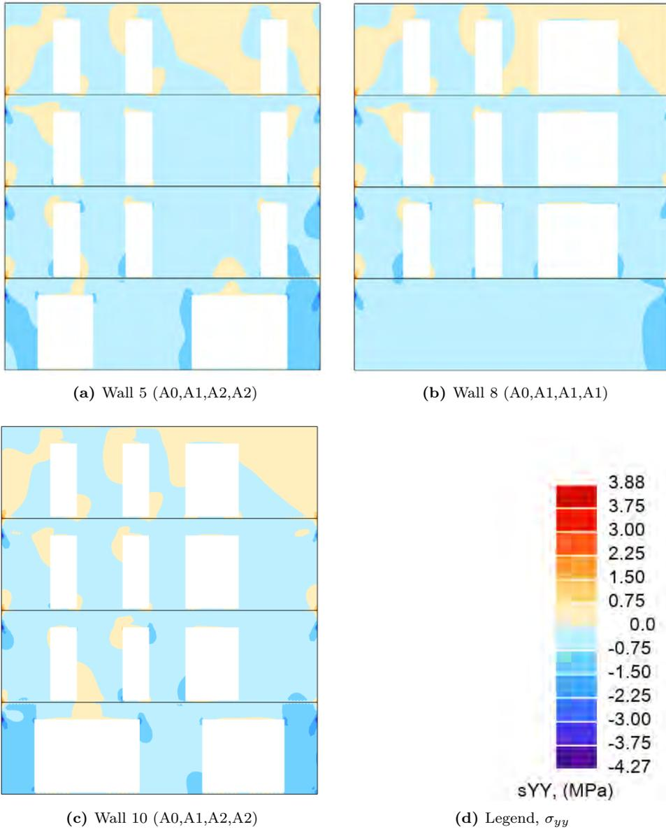
**Figure D.20:** Walls with original opening C and D, new openings. Vertical stresses  $\sigma_{yy}$  [MPa].
