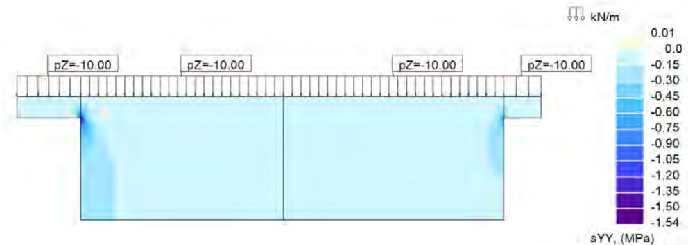
**Figure 4.17:** Illustration of vertical stresses  $\sigma_{yy}$ . Negative blue numbers = compression. Positive orange numbers = tension.
