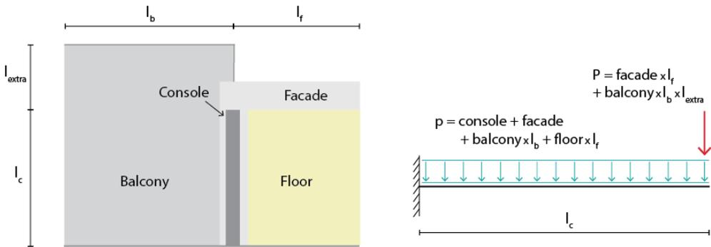
**Figure 4.23:** Illustration of loads for design proposal 2 with facade and balcony, plan view and cantilevered beam.
