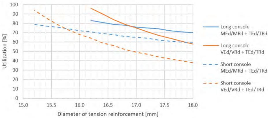
**Figure 4.22:** Utilization of long and short consoles as a function of the diameter of the tension reinforcement.
