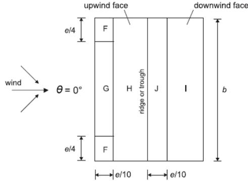
Figure C.7: Wind pressure zones for roof, wind perpendicular to facade [34].
