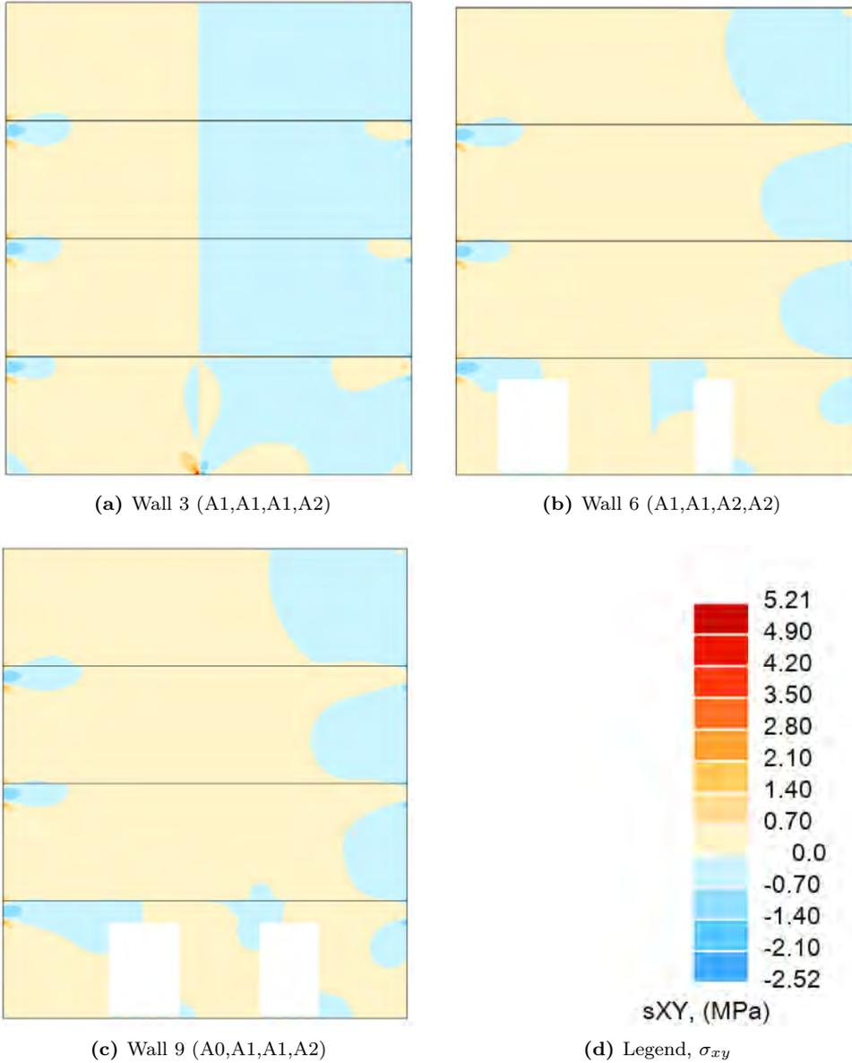
**Figure D.12:** Walls without openings. Shear stresses  $\sigma_{xy}$  [MPa].
