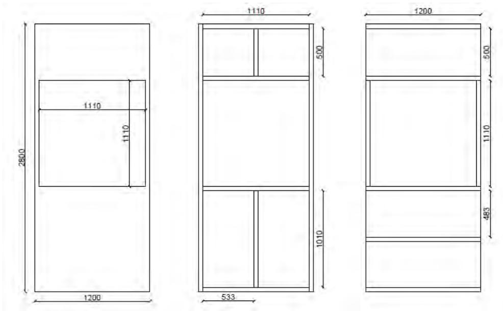
**Figure C.1:** Facade dimensions [mm] for 1.2m element. Wall area, placement of 45x45 timber laths and placement of 200x45mm timber laths.
