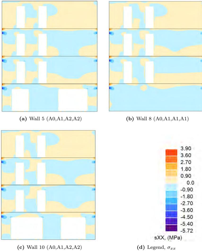
**Figure 4.27:** Walls with opening C and D. Horizontal stresses  $\sigma_{xx}$  [MPa].
