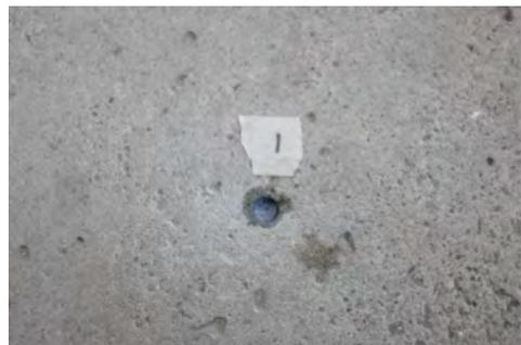
**Figure 3.8:** Carbonation indication with thymolphthalein.
