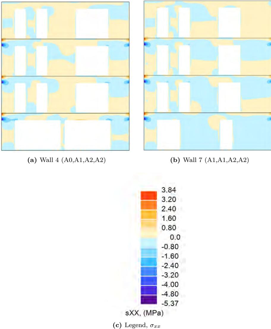
**Figure D.16:** Walls with original opening A and B, new openings. Horizontal stresses  $\sigma_{xx}$  [MPa].
