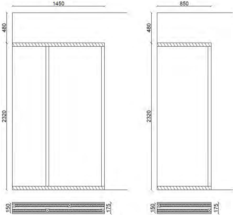
**Figure C.3:** Inner wall for a long and short console [mm].
