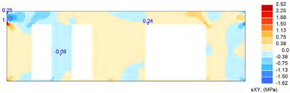
**Figure 4.40:** Shear stresses  $\sigma_{xy}$  [MPa] in wall 4, level 1, with extra load from new floor.
