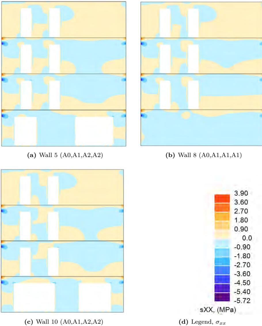
**Figure D.4:** Walls with opening C and D. Horizontal stresses  $\sigma_{xx}$  [MPa].
