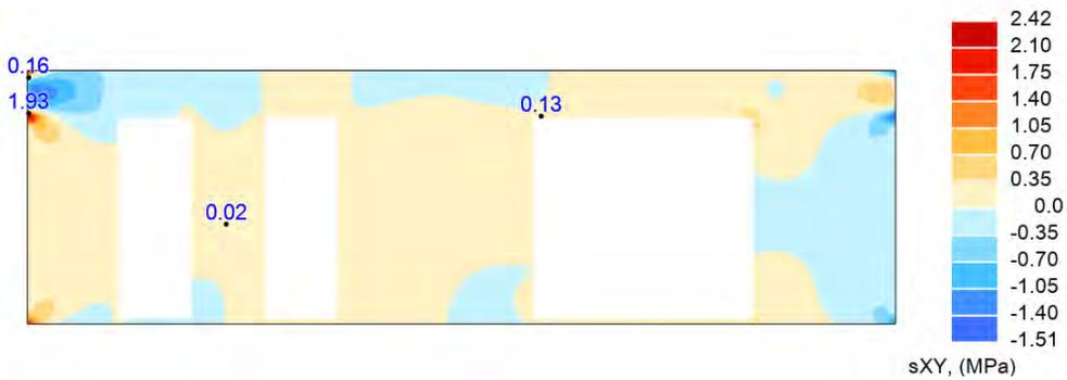
**Figure 4.37:** Shear stresses  $\sigma_{xy}$  [MPa] in wall 4, level 1, with new openings.
