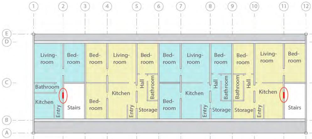
**Figure 4.8:** Proposal - new openings in bearing walls.
