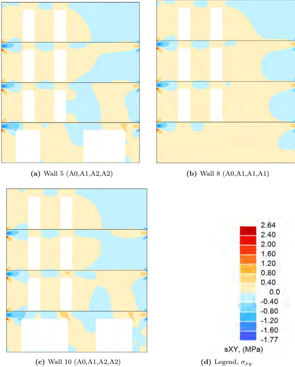
**Figure D.6:** Walls with opening C and D. Shear stresses  $\sigma_{xy}$  [MPa].
