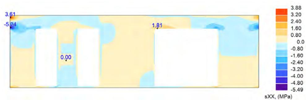
**Figure 4.38:** Horizontal stresses  $\sigma_{xx}$  [MPa] in wall 4, level 1, with extra load from new floor.
