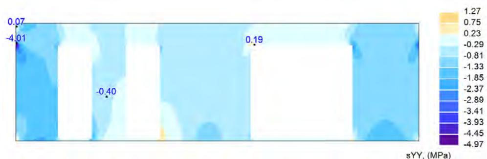
**Figure 4.39:** Vertical stresses  $\sigma_{yy}$  [MPa] in wall 4, level 1, with extra load from new floor.
