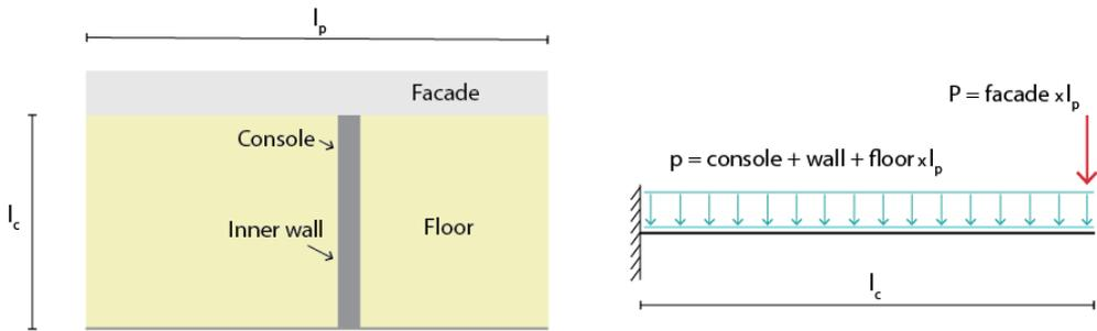
**Figure 4.21:** Illustration of loads for design proposal 2 with a facade, plan view and cantilevered beam.
