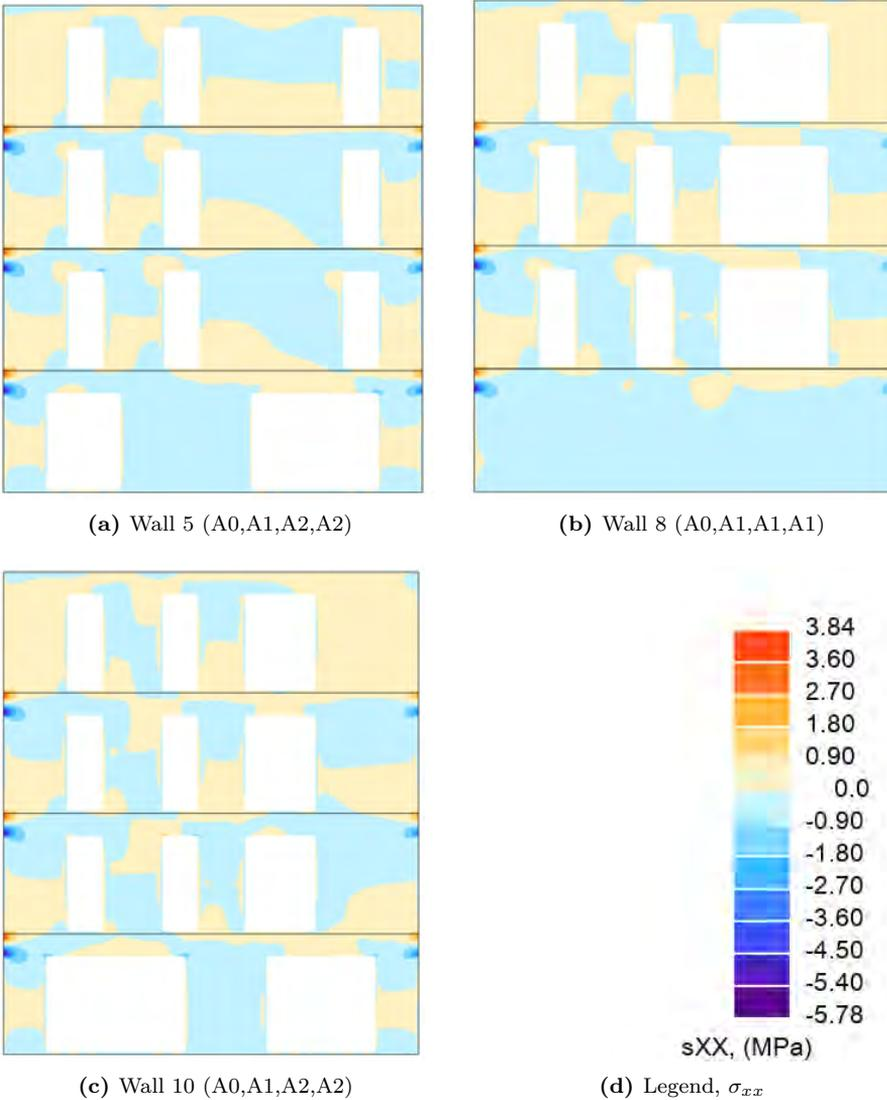
**Figure D.19:** Walls with original opening C and D, new openings. Horizontal stresses  $\sigma_{xx}$  [MPa].
