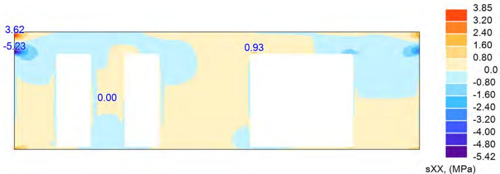
**Figure 4.35:** Horizontal stresses  $\sigma_{xx}$  [MPa] in wall 4, level 1, with new openings.
