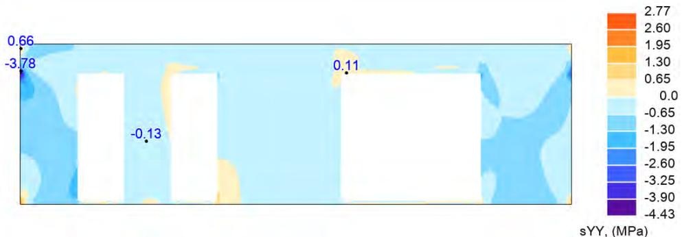
**Figure 4.36:** Vertical stresses  $\sigma_{yy}$  [MPa] in wall 4, level 1, with new openings.
