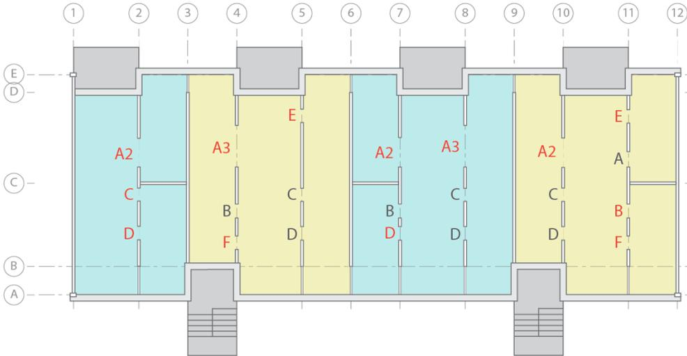
**Figure 4.32:** Illustration of existing and new openings in walls. New openings are marked with red.
