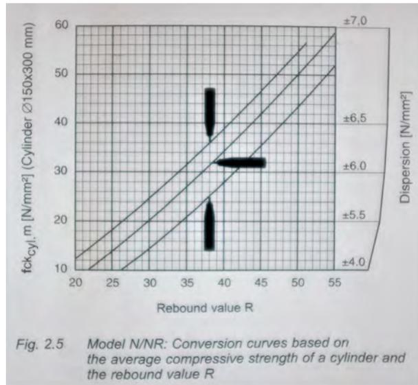
**Figure B.1:** Schmidt Hammer conversion curve [21].
