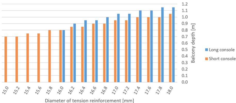
**Figure 4.24:** Extra depth of balcony compared to diameter of tension reinforcement.
