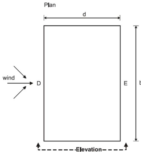
**Figure C.4:** Zones for wind pressure coefficients, plan view [34].
