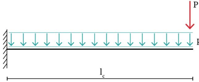
**Figure 4.12:** Uniform load  $p$  and point load  $P$  on cantilevered beam.
