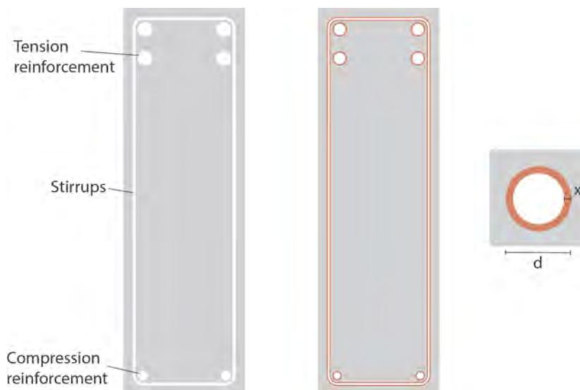
**Figure 4.11:** Cross section of a long console with un-corroded and corroded reinforcement.
