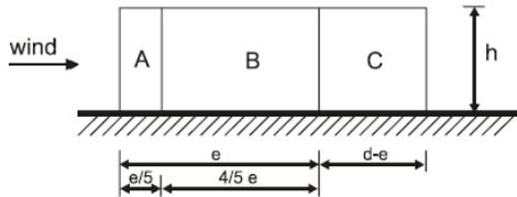
**Figure C.6:** Wind pressure zones for vertical walls,  $e \leq d$  [34], wind perpendicular to gable.
