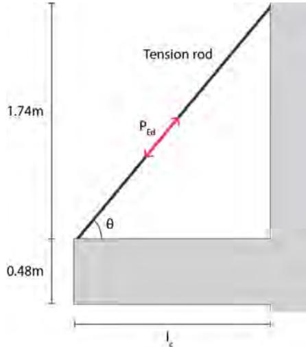
**Figure 4.26:** Inclined tension rod attached between a console and the bearing wall.
