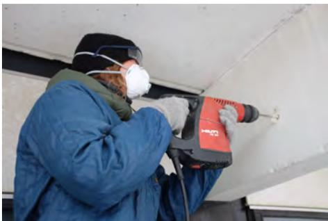
**Figure 3.7:** Drilling of holes for carbonation test.
