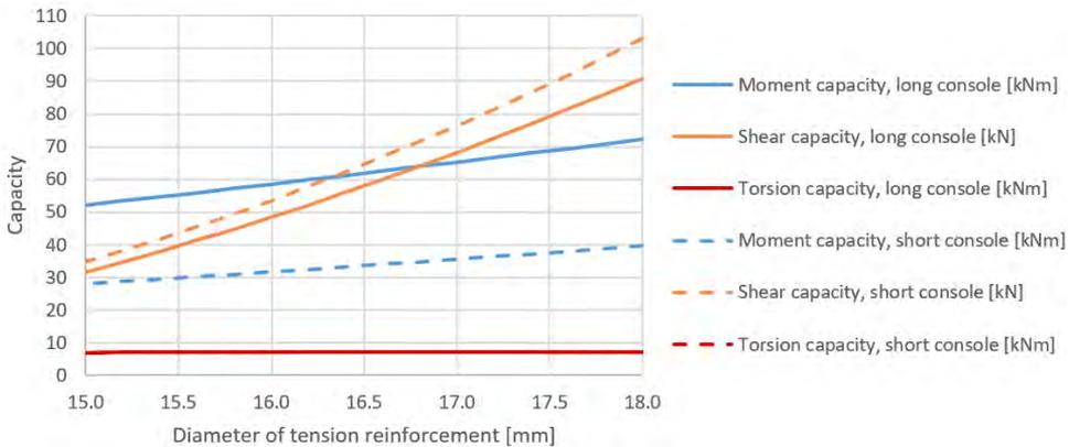
**Figure 4.19:** Moment, shear and torsion capacity for a long and short console compared to the diameter of the tension reinforcement.
